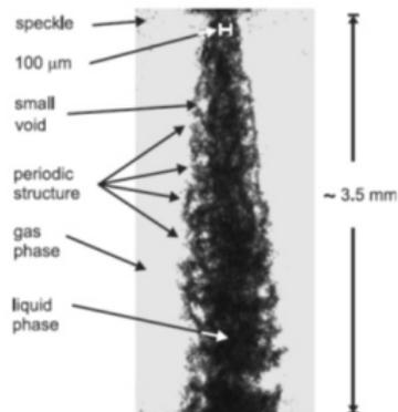
CSM<sup>§</sup>, Diesel fuel spray into 1 atm at  $We = 7.6 \times 10^5$  &  $Re = 1.6 \times 10^4$
